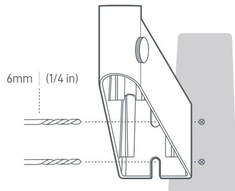
**7 | Apply Sealant and Screw in Wall Mount**
