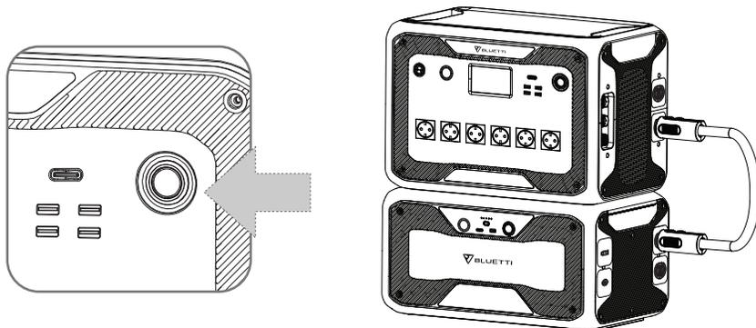
**Note:** Please connect the AC300 and B300 with the Battery Expansion Cable.
