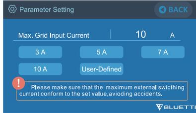
**Note:** The Grid Input Current is set at 10A by default. The change only takes effect when AC300 connects to the grid.
