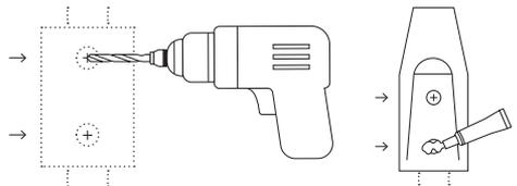
4. Place mount over holes and insert screws. Use the drill with socket to drive screws in 90%; do not overdrive. Use socket wrench to tighten screws plus ¼ turn; do not overtighten.
